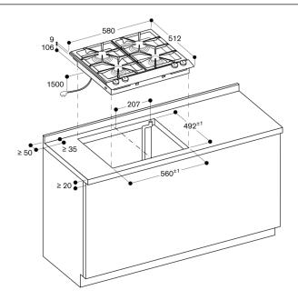
Minimum distance from the appliance cut-out to the side wall 150 mm.
