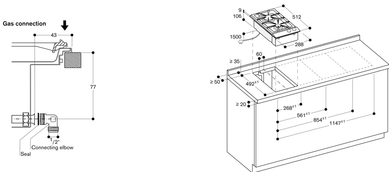
Minimum distance from the appliance cut-out to the side wall 150 mm.
