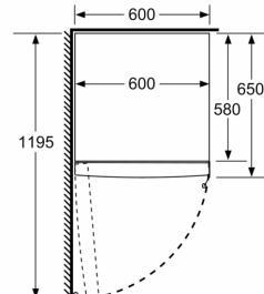
measurements in mm
