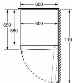
measurements in mm
