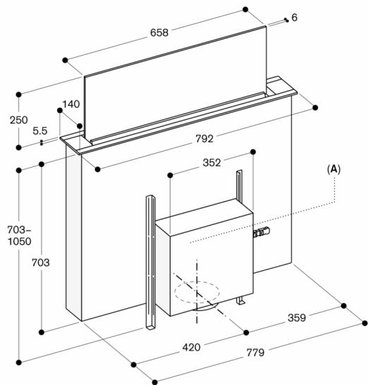
A: Flexible installation of the fan unit at the front, at the back or at a distance from the appliance (installation kit required - max. distance 3 m)
