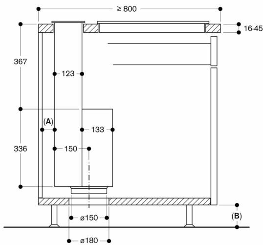
**A:**  $\geq 20$  mm from the Guided Air suction area to a cabinet wall
