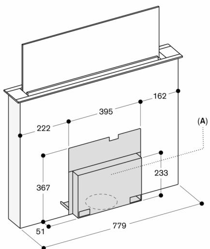
**A:** Access to the complete cover must be ensured even after installation
