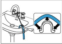
Fix and secure the water outlet hose with an elbow.
