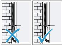
Do not trap the power cord or the hoses between the wall and the appliance.
