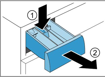
3. Pull out the insert upwards.
