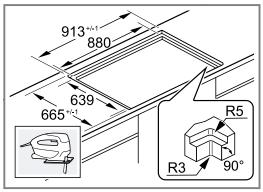
The angle between the cut surface and the worktop must be  $90^{\circ}$ .
