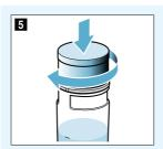
5 Press the lid of the water tank down and screw it back on.
